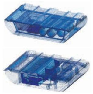
Complex meshes of different traction components generated by ANSYS ICEM CFD meshing software
